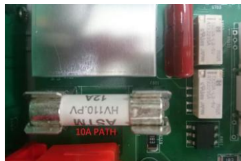
Internal 10A input current fuse
