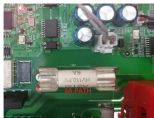
Internal 3A input current fuse
