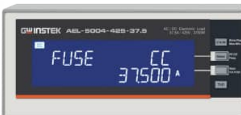
Turbo : OFF, Fuse mode Test result screen
