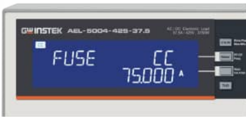
Turbo ON, Fuse mode Test result screen
