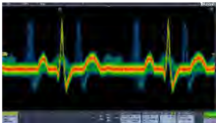
Digital phosphor technology with FastAcq enables greater than 280,000 wfms/s waveform capture rate and real-time color-intensity grading.
