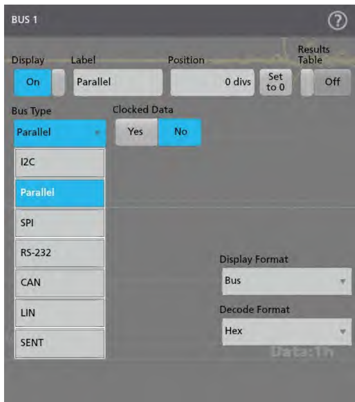
Bus menu provides options to configure the bus parameters
