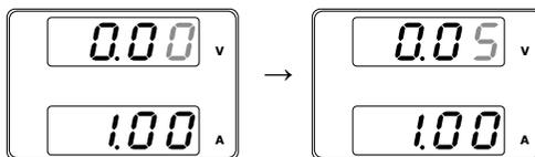
3. Repeatedly press the Voltage knob until the first digit is highlighted. This will allow the voltage to be edited in 1 volt steps.
