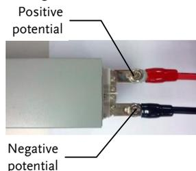
Connection with voltage sense wiring
