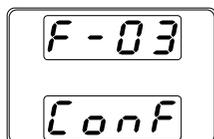
6. If CV Slew Rate Priority was chosen as the operating mode, repeat steps 3~5 to set F-04 (Rising Voltage Slew Rate) and the F-05 (Falling Voltage Slew Rate) and save.
