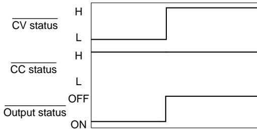
CC MODE: The diagram below shows the timing diagram when the output is turned on when the PRP is set to CC mode.
